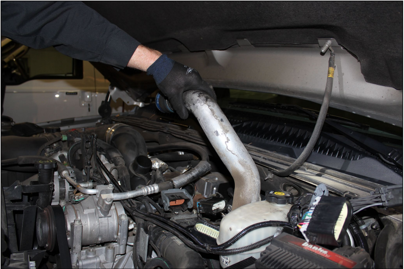
FIGURE 6 – REMOVING THE DRIVER SIDE INTERCOOLER TUBE
