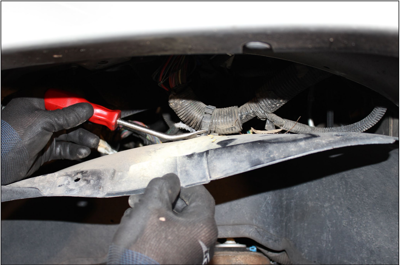
FIGURE 2 – RELEASING WIRING HARNESS BEFORE REMOVING INNER FENDER
