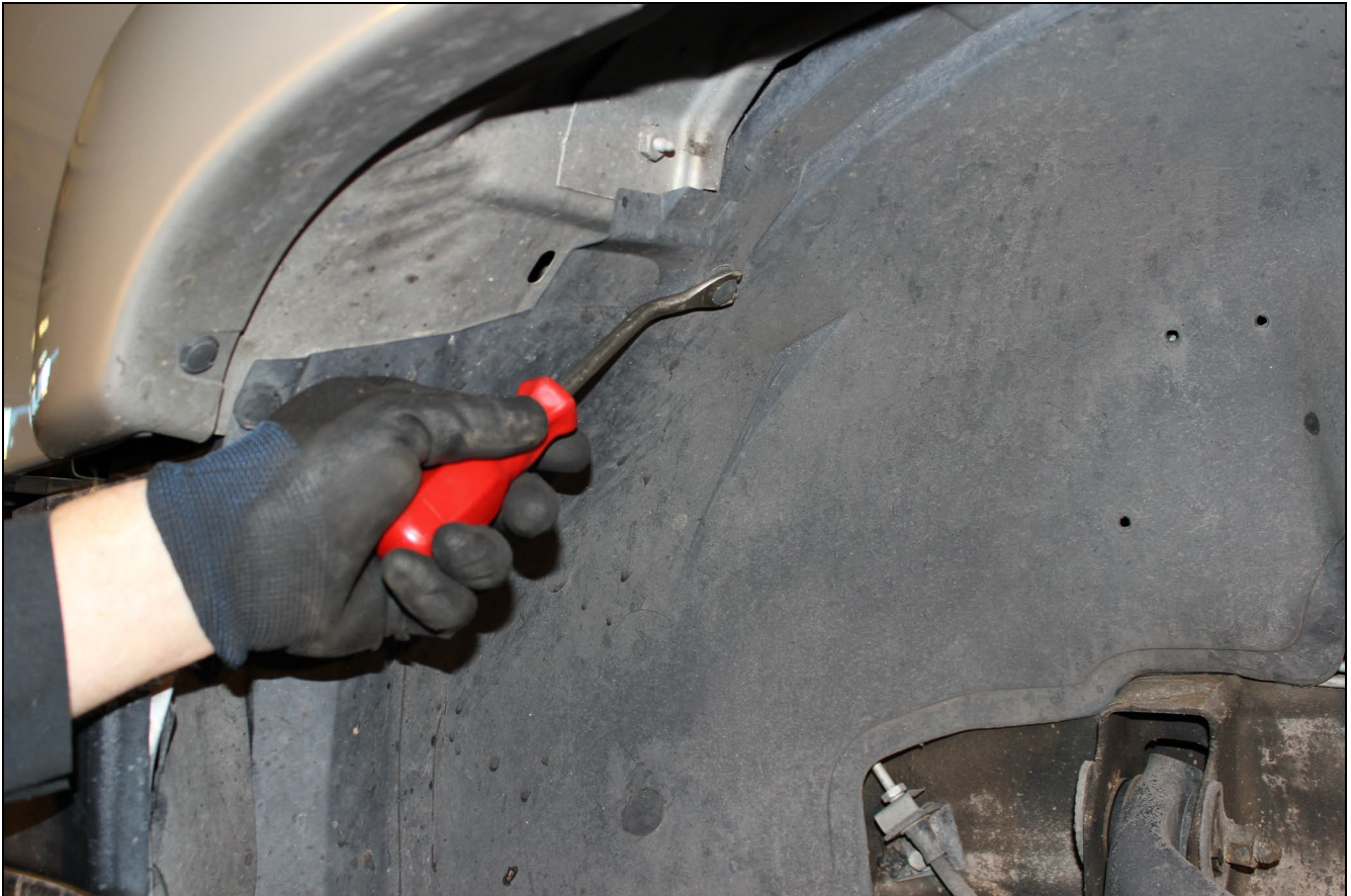
FIGURE 1 – REMOVING INNER FENDER RETAINER CLIPS
