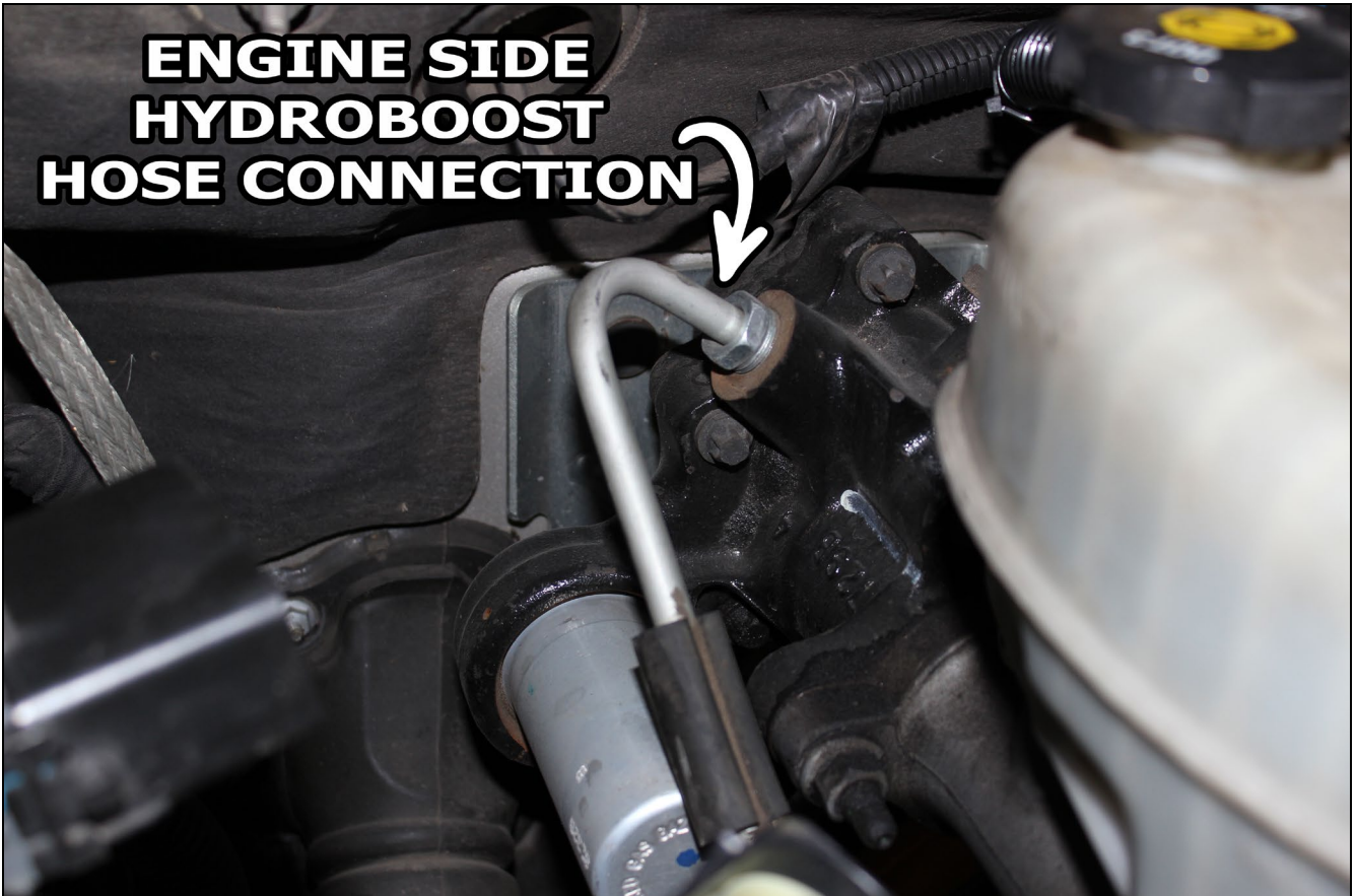
FIGURE 11 – ENGINE SIDE HYDROBOOST HOSE/TUBE CONNECTION
