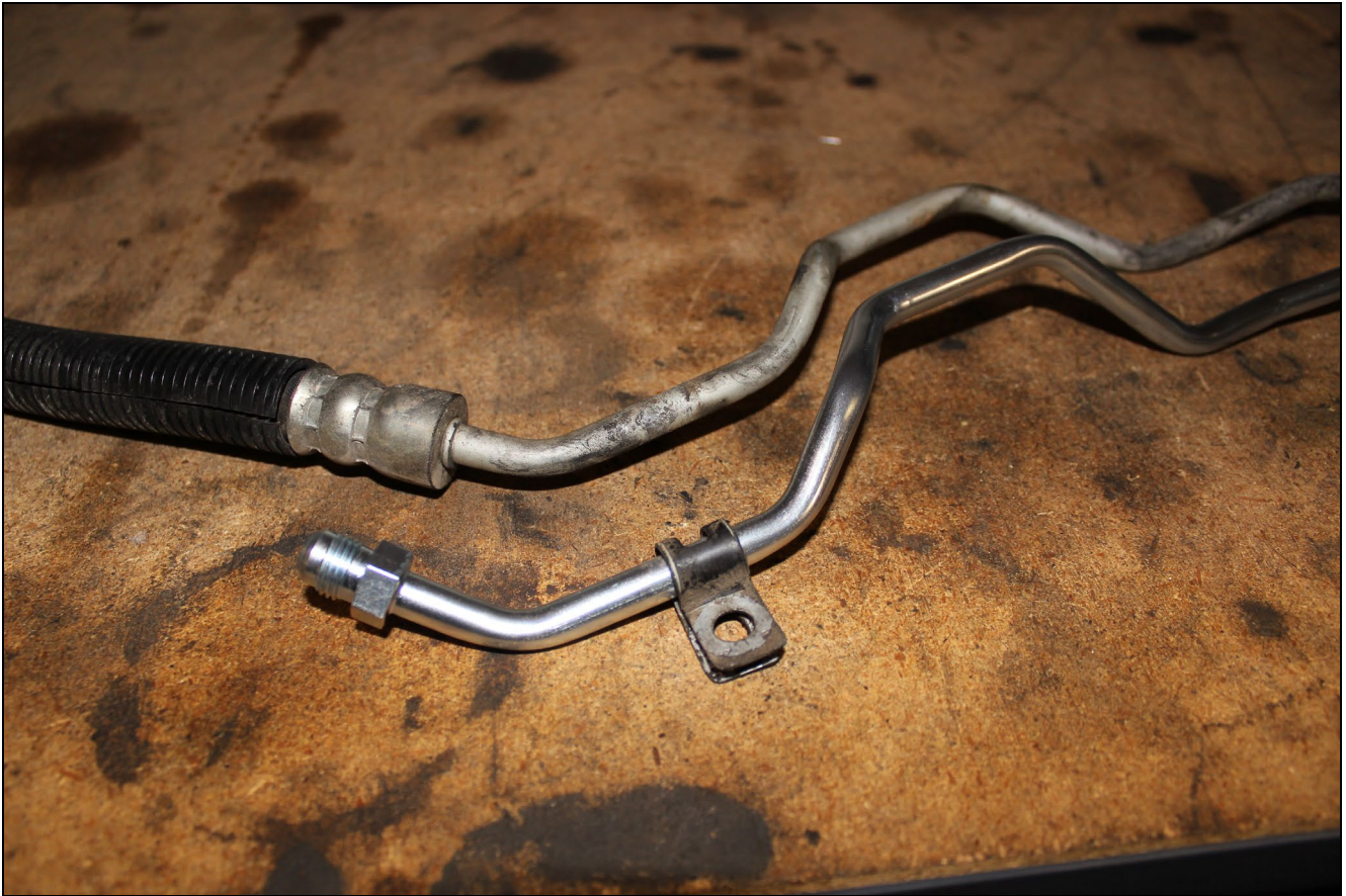
FIGURE 14 – CORRECT ORIENTATION OF TRANSFERRED TUBE CLAMP – IMPORTANT!
