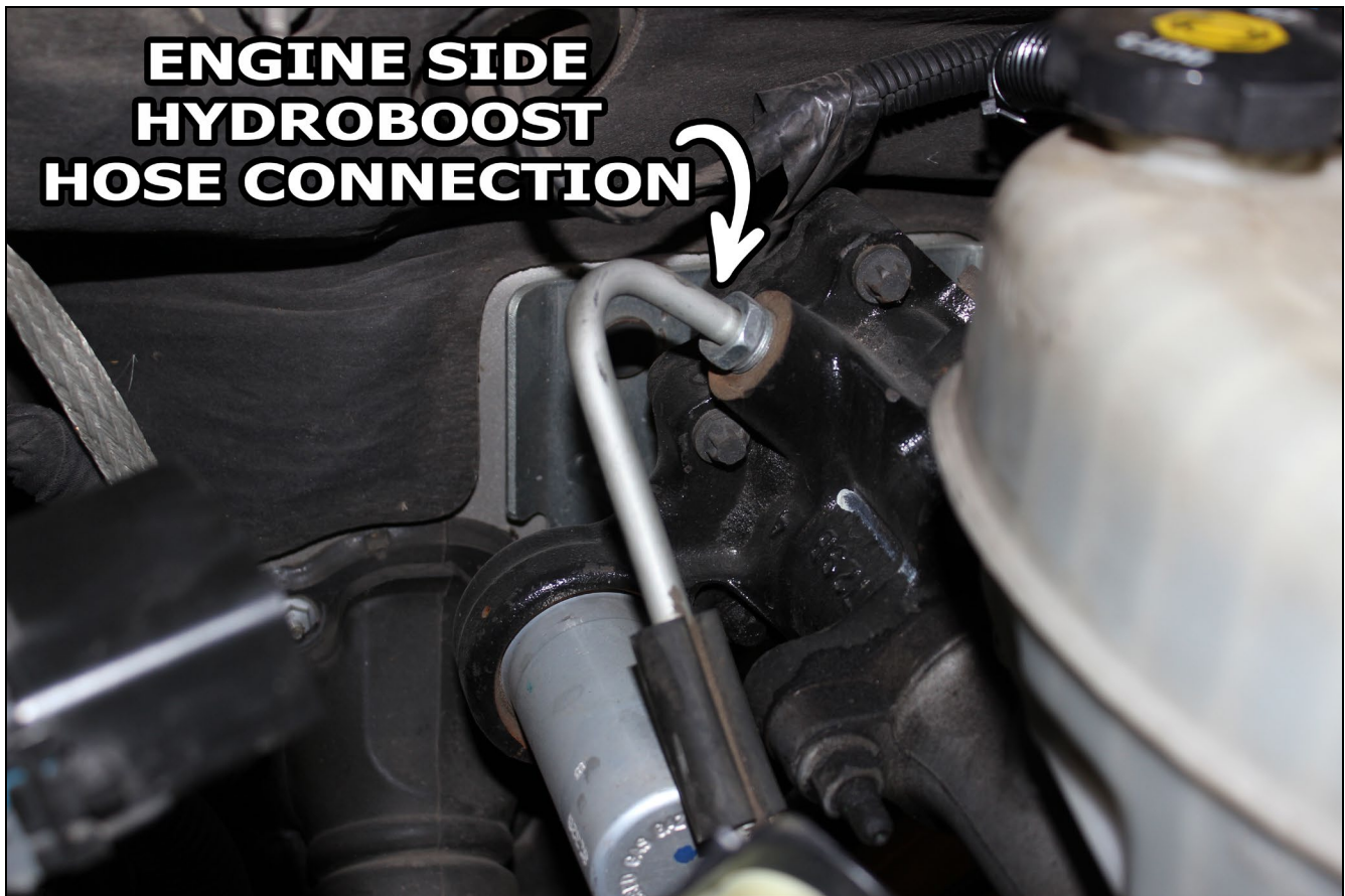
FIGURE 11 – ENGINE SIDE HYDROBOOST HOSE/TUBE CONNECTION
