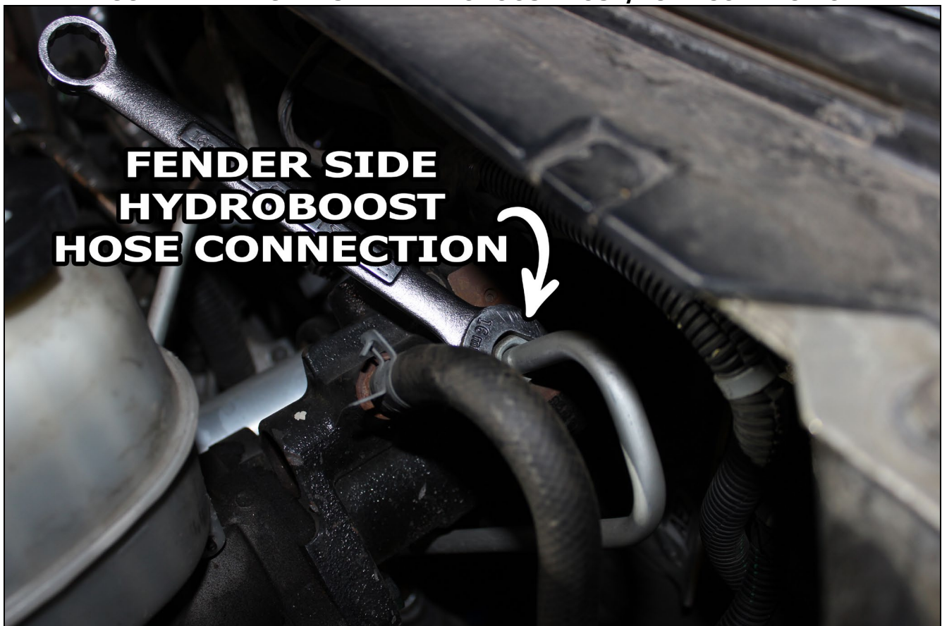
FIGURE 12 – FENDER SIDE HYDROBOOST HOSE/TUBE CONNECTION
