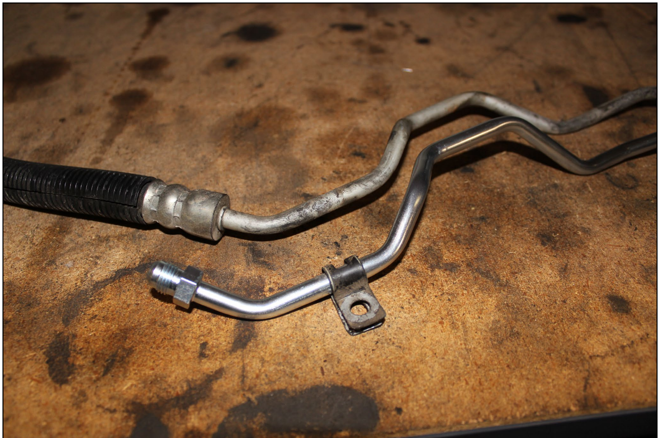
FIGURE 14 – CORRECT ORIENTATION OF TRANSFERRED TUBE CLAMP – IMPORTANT!
