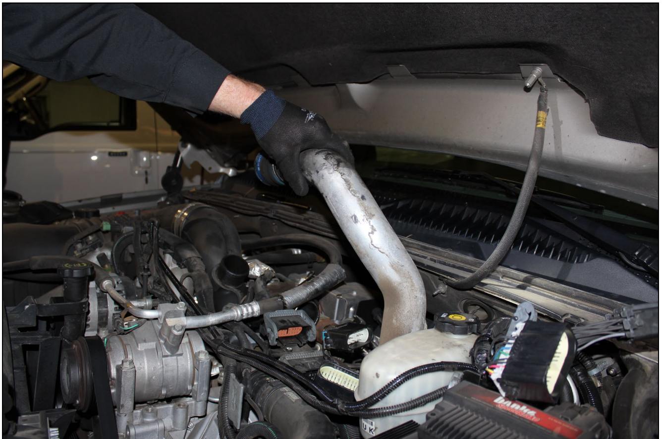
FIGURE 6 – REMOVING THE DRIVER SIDE INTERCOOLER TUBE
