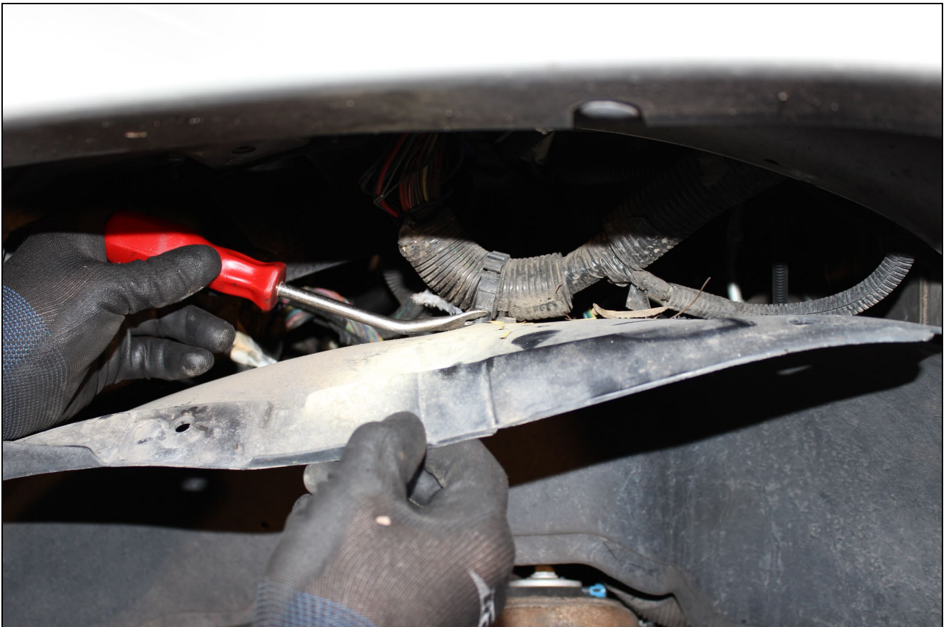
FIGURE 2 – RELEASING WIRING HARNESS BEFORE REMOVING INNER FENDER
