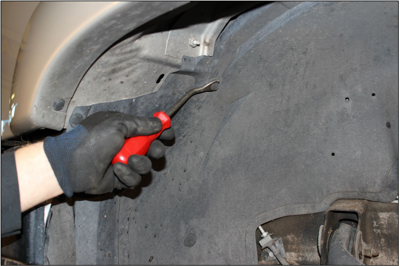
FIGURE 1 – REMOVING INNER FENDER RETAINER CLIPS
