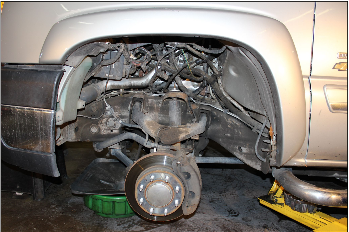
FIGURE 3 – INNER FENDER REMOVED
