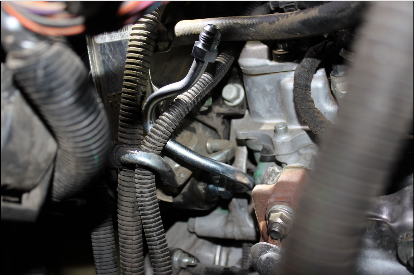
FIGURE 15 – CORRECT ORIENTATION OF THE POWER STEERING PUMP TUBE
